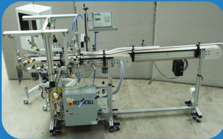
Leak Detector System with Vision Inspection
