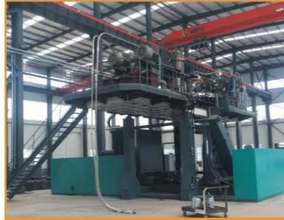
Pet All's biggest Jumbo-series machine is capable of producing parts with a volume of up to 25,000 liters.
