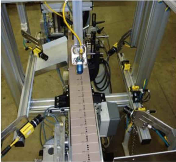
Camera System: Close-up showing 4 X 1200 & LED overhead illumination light
